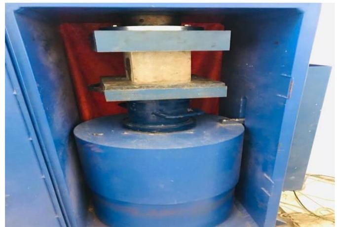
Fig. 4.2.1UTM for compressive strength test
