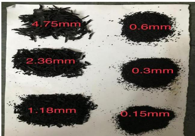
**2.4 Fine Aggregate:-**FA are locally accessible. All the Experiments that were operated on CA are according to IS: 383-1970.
