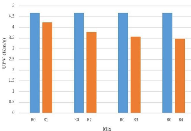
**Fig. 4.2.13** UPV of RMSCC compared with SCC
