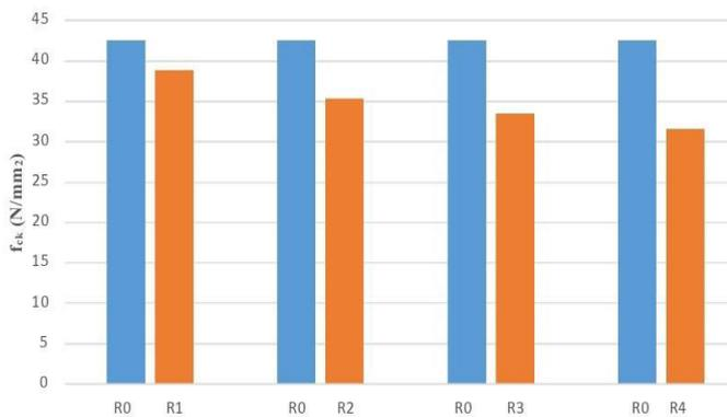
Fig. 4.2.3 fck of RMSSC compared with SCC after 28 days of curing
