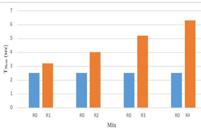
Fig.4.1.3 T50cm time of RMSCC compared with SCC
