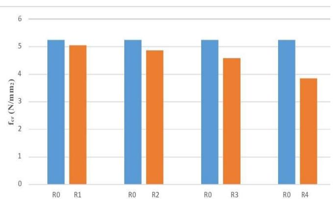
Fig. 4.2.6 fcr of RMSSC compared with SCC after 28 days of curing
