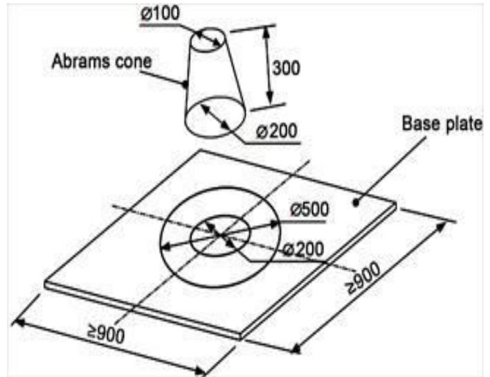
**Fig. 4.1.1 Schematic diagram of slump cone and base plate**
