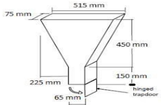
Fig. 4.1.3 Schematic diagram of V-Funnel apparatus
