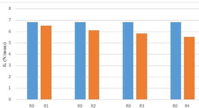
Fig. 4.2.9 fb of RMSCC compared with SCC after 28 days of curing
