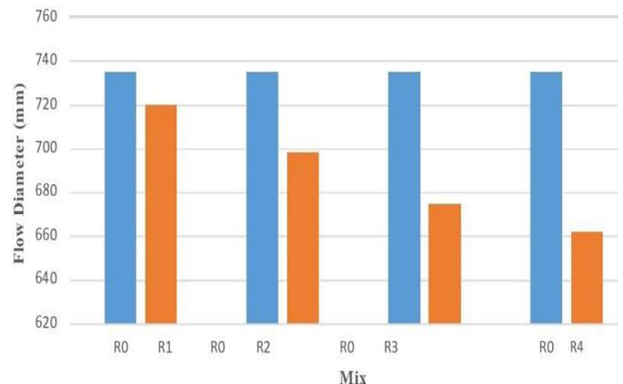
**Fig.4.1.2 Flow diameter of RMSCC compared with SCC**
