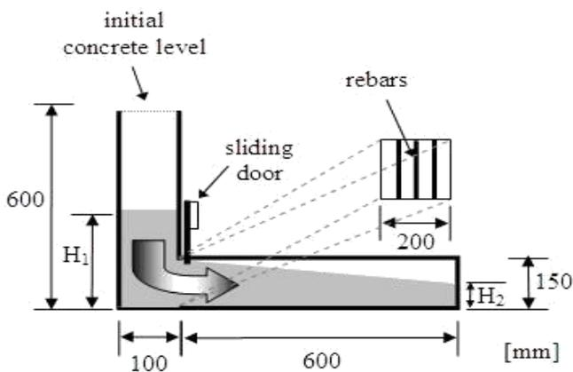
Fig. 4.1.4 Schematic diagram of L-Box apparatus
