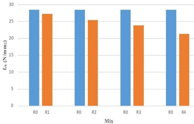
Fig. 4.2.2 fck of RMSSC compared with SCC after 7 days of curing
