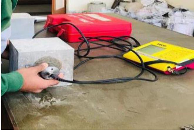
**Fig. 4.2.12** Performing ultrasonic pulse velocity test
