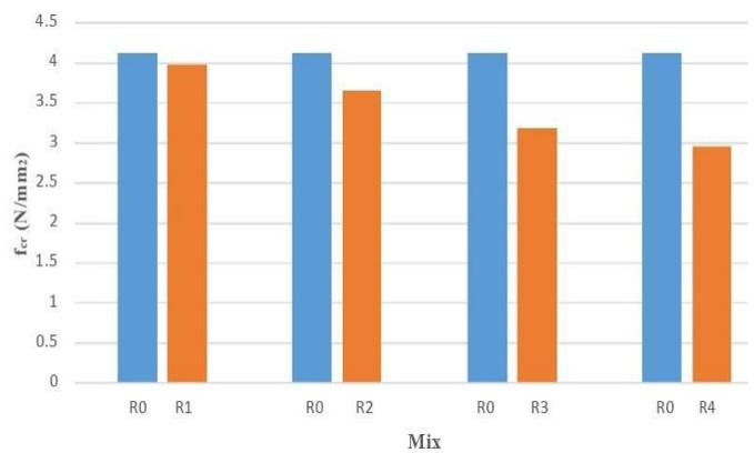
Fig. 4.2.5 fcr of RMSSC compared with SCC after 7 days of curing
