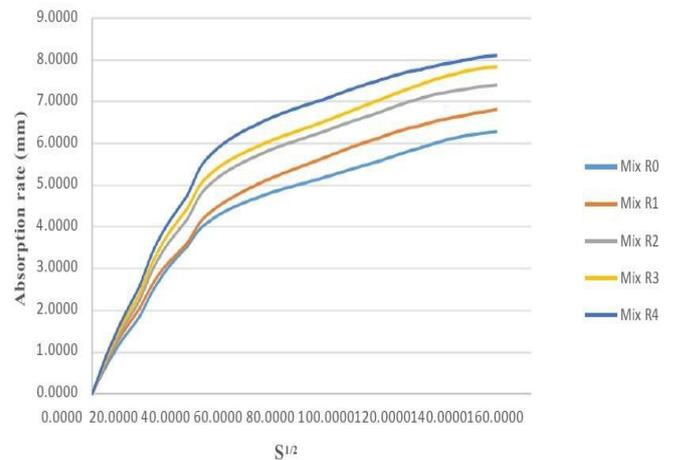
Fig. 4.2.11 Variation of absorption rate vs square root of time for all mixes of SCC
