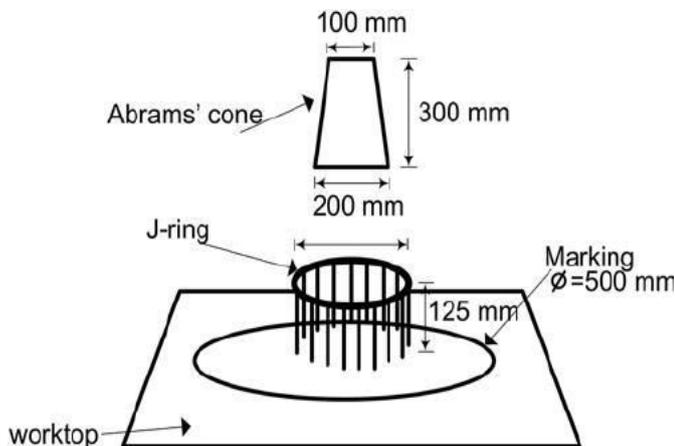
Fig. 4.1.4 Schematic diagram of slump cone and J-Ring apparatus
