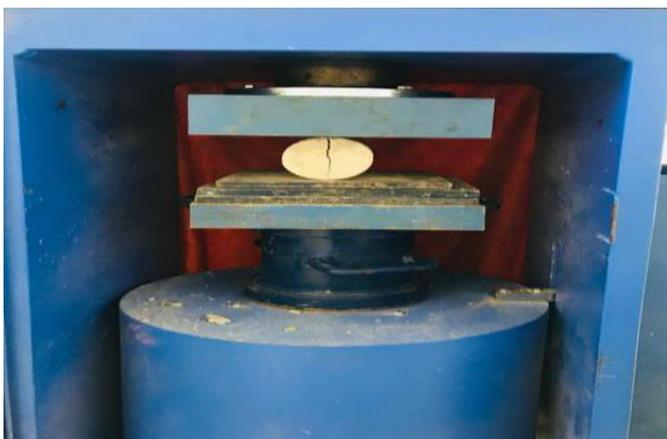
Fig. 4.2.4 UTM for splitting tensile strength test
