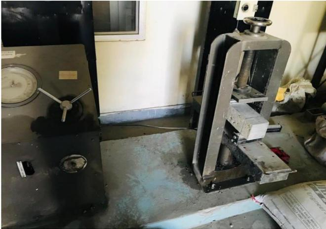
Fig. 4.2.7 Flexural tensile strength apparatus
